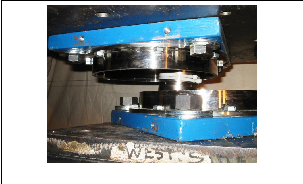
Figure 4. Photograph of the bearing at maximum displacement
