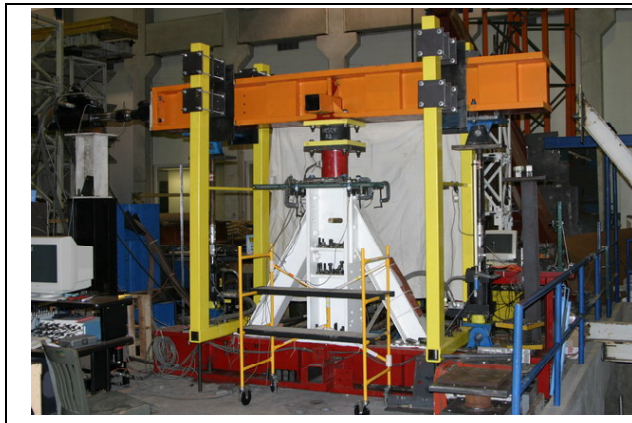
Figure 2. Small bearing testing machine
