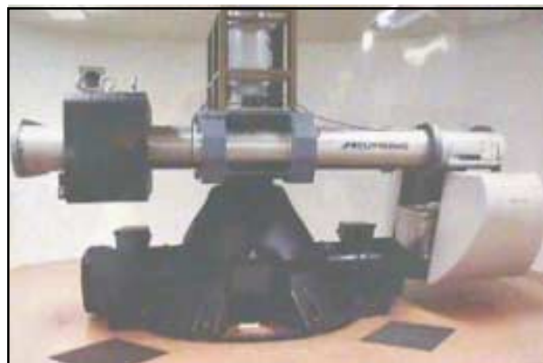
■ Figure 2. 100 g-ton geotechnical centrifuge with in-flight shaking capability at RPI
