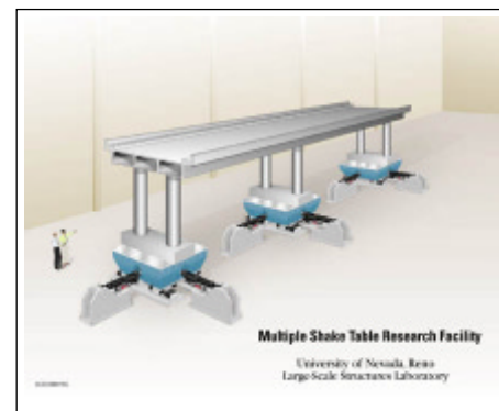
■ Schematic realization of the multiple shake table facility at the University of Nevada, Reno.
