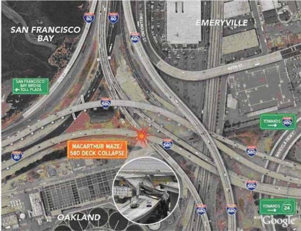
Figure 2.2.1. Aerial Photo of Collapsed Portion of MacArthur Maze
