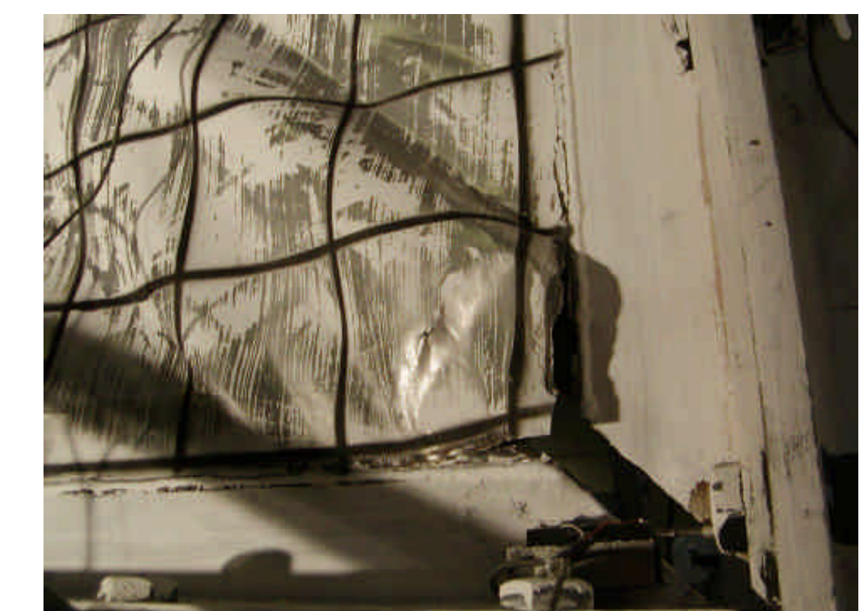
Figure 10 Specimen F2 Infill Fractures 10d
