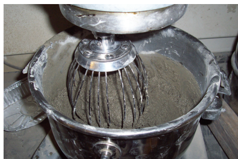
Fig. 10. Standard table mixer and microconcrete mix.
