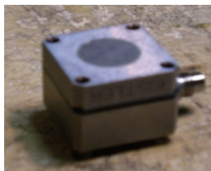
Figure 12, accelerometer at -1 g (Rooney, 2007)
