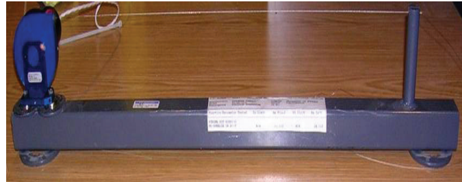
Figure 10, string pot calibration length (Weinreber, 2007)
