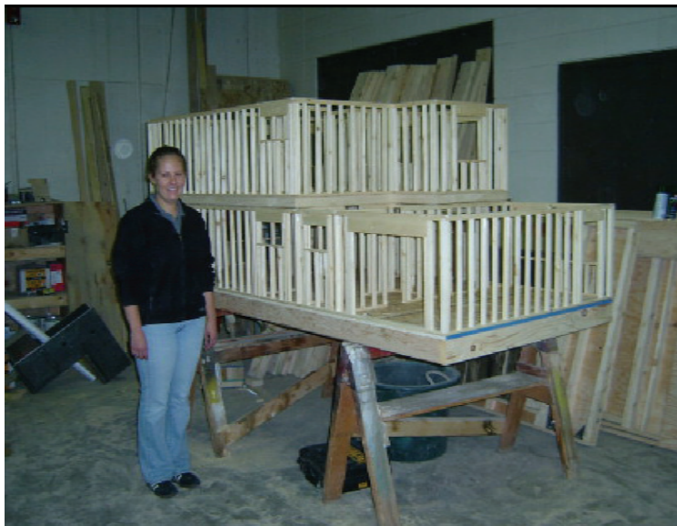
Figure 1. 1:6 Scale Model House in Construction
