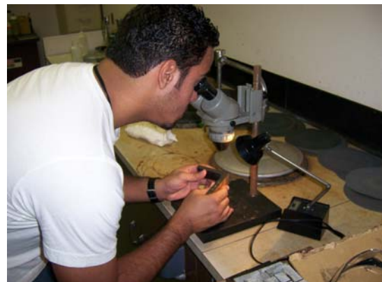
Figure 21: Visualizing welded sections
