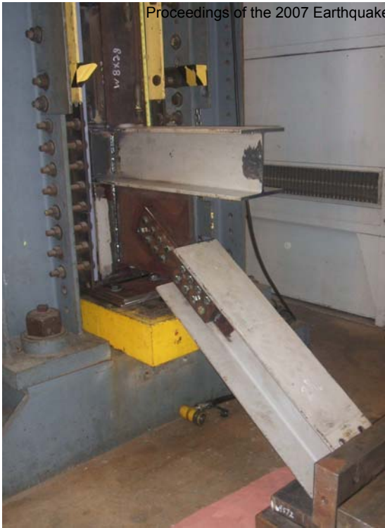
Figure 11: Connection Specimen in drop hammer machine.
