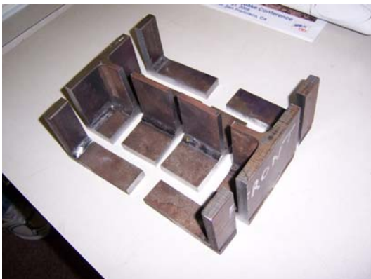
Figure 20: Sliced bottom part of the column stub
