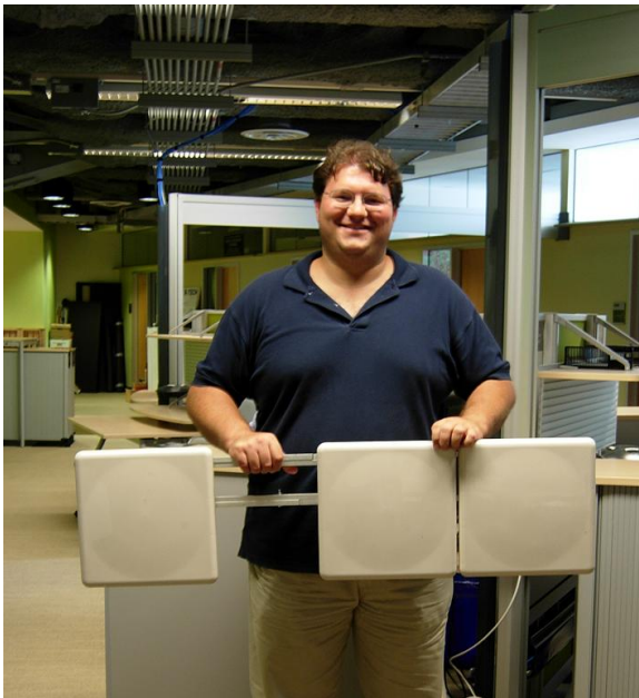
Figure 11: The assembled array. Note the asymmetrical assembly of the antennas.
