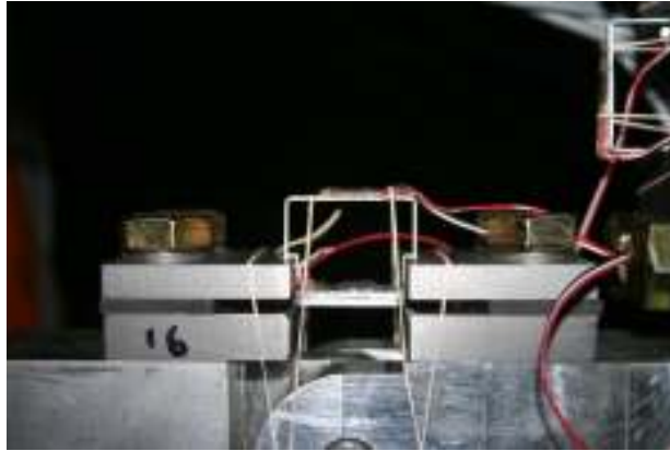
Figure 7: Homemade clip gauge
