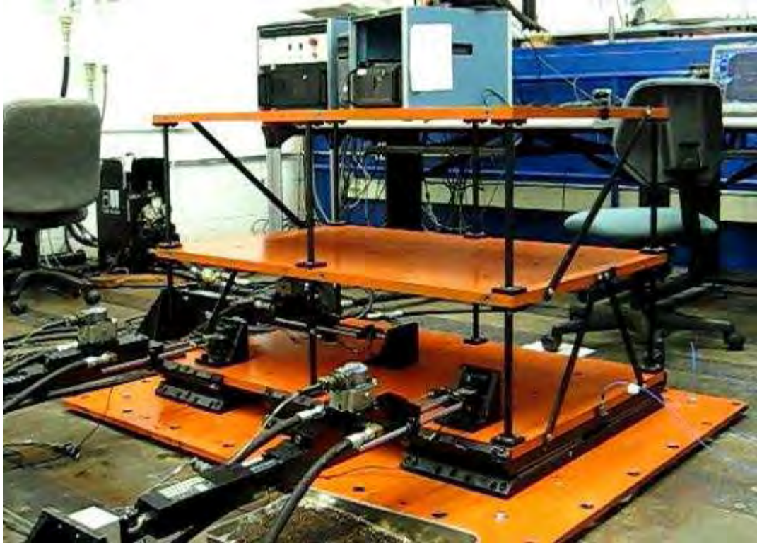
Figure 2: Picture of test structure during system identification stage
